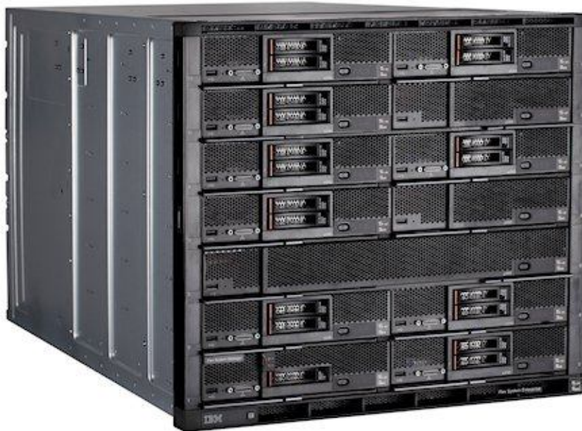
Figure 1. The IBM Flex System Enterprise Chassis
